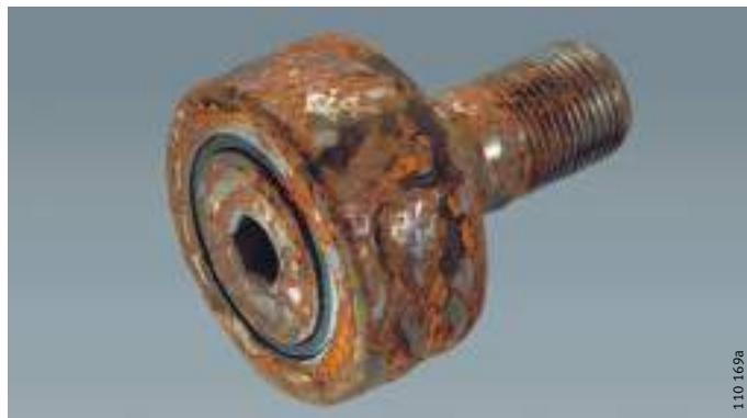
Figure 26 NUKR52 without plating after salt spray test
