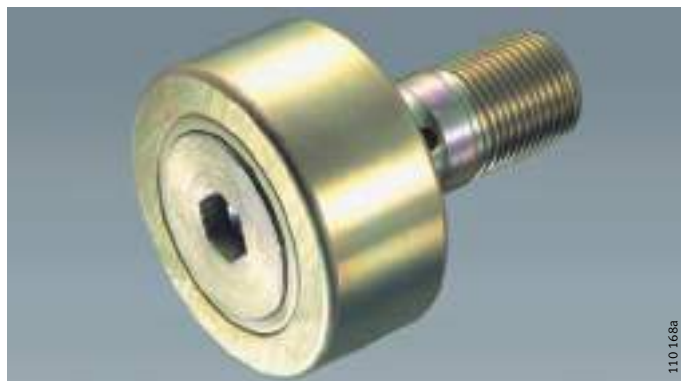
Figure 27 PWKR52-2RS-RR with Corrotect® plating after salt spray test
