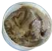
Used grease: colour turned greyish
